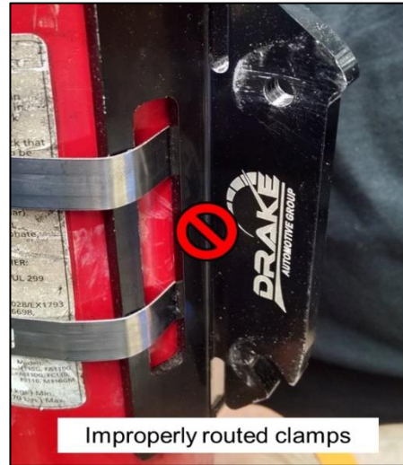
Image B-44.3: Fire Extinguisher, Incorrect routing of hose clamps
