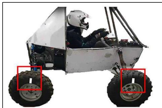
Image F-1: Tire Markings for Wheel Lock Check
