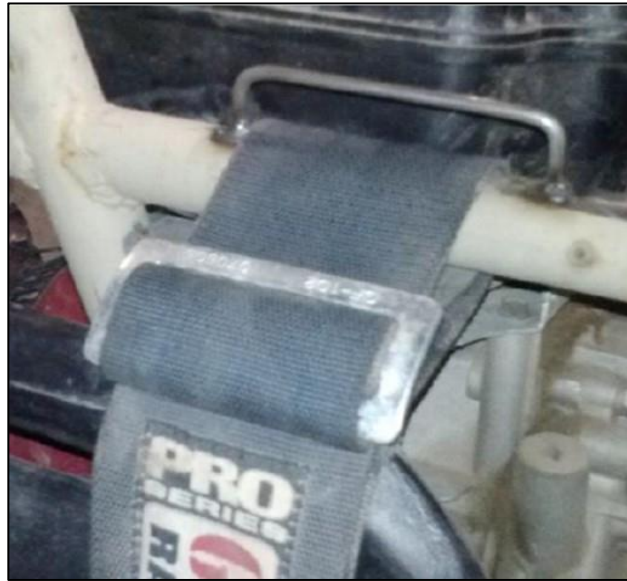
Image B-33: Driver Harness, Shoulder Harness, Lateral Restraint
